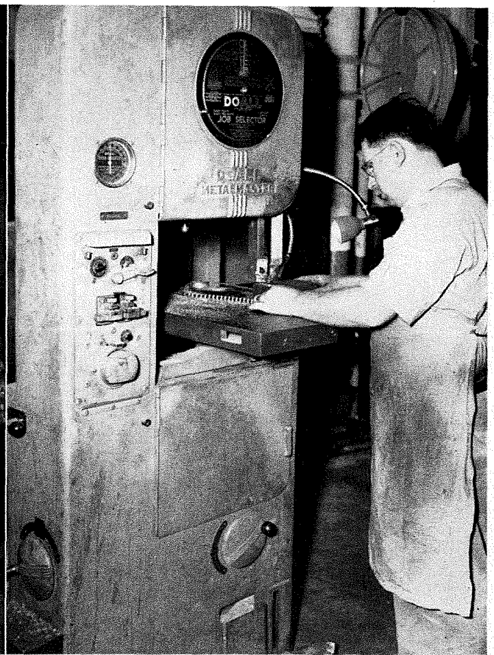
Toolmaker RICHARD HUSTON contour saws a 2 1/8" steel blanking die on a DoAll Model ML. The controls to the left of the sawing area are for the built-in welding machine. The saw blade is continuous, therefore, the ends must be welded together.
